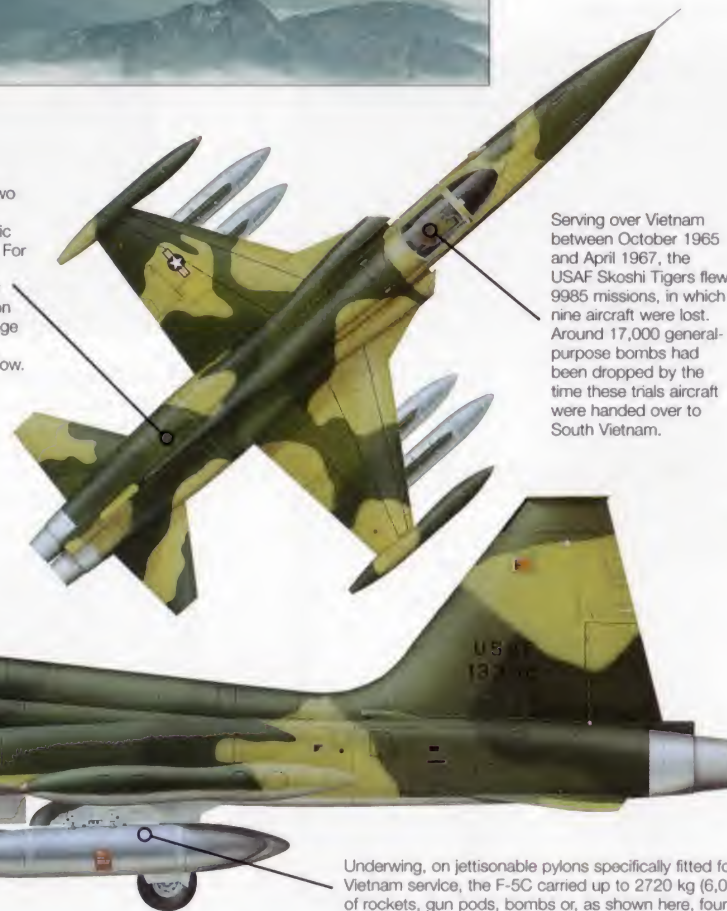
For long-range missions, the Freedom Fighter's wing-tip missile pylons can be replaced with fuel tanks.
